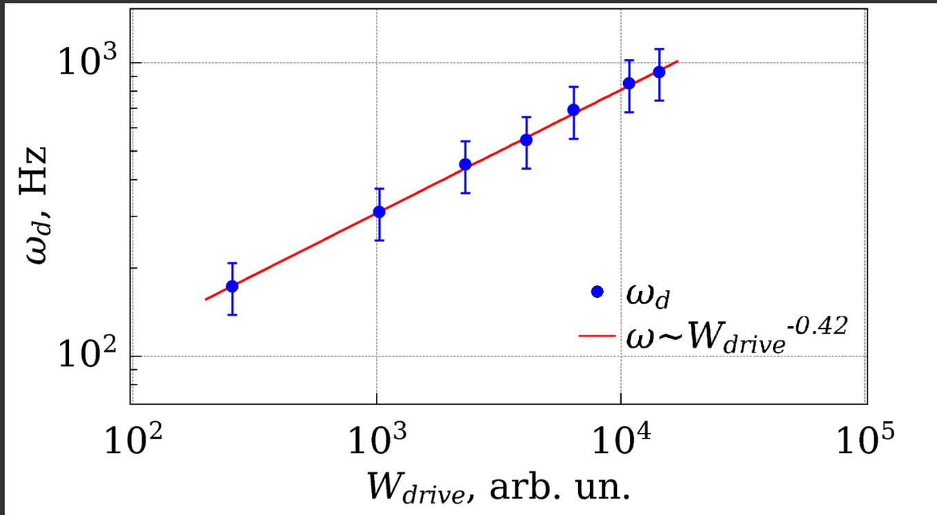
The decay exponent  $\omega_d$  (blue points) as a function of external force power  $W$  is fitted well by power-law  $\omega_d \sim W^{0.4 \pm 0.1}$  (red line).
