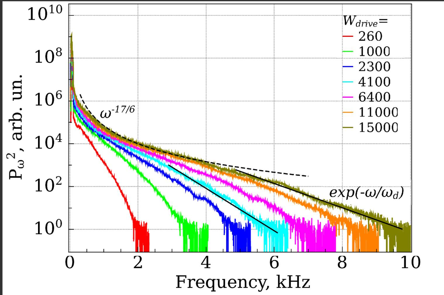
Experimental spectra of surface oscillation  $P_\omega^2$  in semi-logarithmic scale. The high frequency part of spectrum  $P_\omega^2$  can be approximated well by exponential decay.
