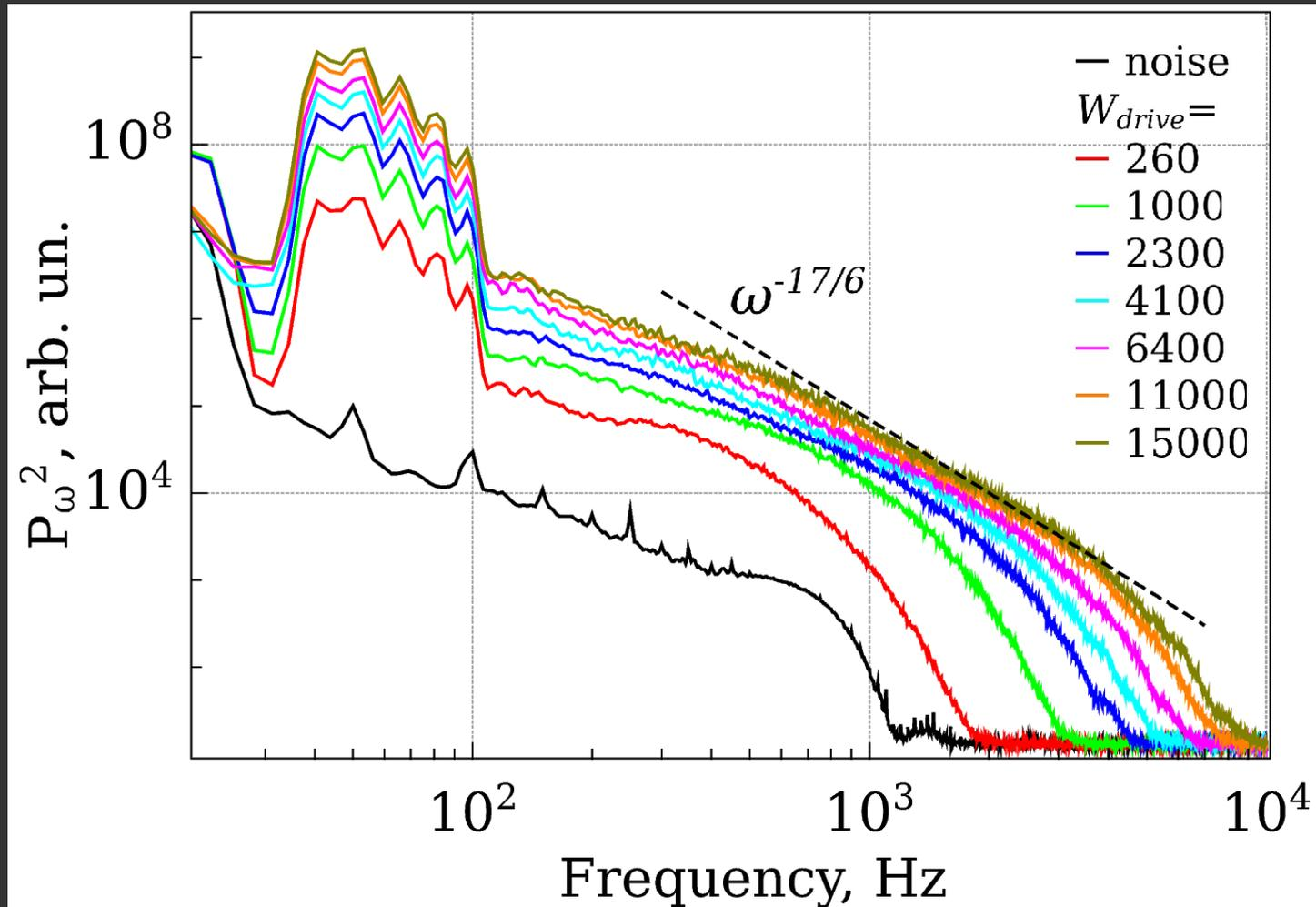
Experimental spectra of surface oscillation  $P_{\omega}^2$  in logarithmic scale. Waves have been excited by external random force in a frequency range 39—103 Hz. Straight segments of the spectra correspond to power-law distribution inside inertial interval.
